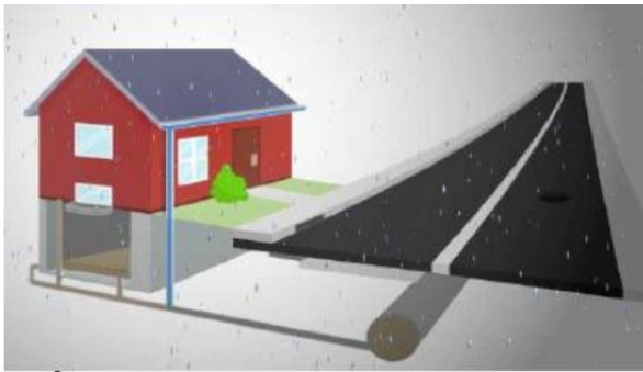
Combined sewer systems have one pipe.
